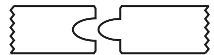
END MATCH All of our decking is end-matched for ease and improved quality of installation and to provide full coverage on or off the joist. Learn more at dassoXTR.com .
